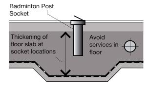
Fig 6: Typical section through sports floor construction
